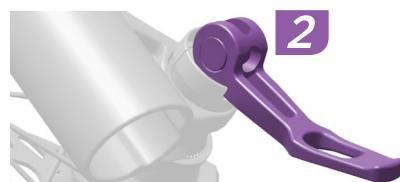
Thread the Maxle into the fork leg by hand and tighten it until it stops.
